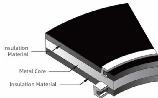
The **PRO-Max** flange isolating gasket kit is usually made of G10 /G11 and SS316 metal core, and it provides exceptional insulating and general sealing performance in aggressive material applications. The **PRO-Max** flange isolating gasket kit is suitable in all very critical services up to and including ANSI 2500# and API 10,000# classes. And it can match all types of flanges such as raised flange, full face flanges, Ring type joint flanges.
