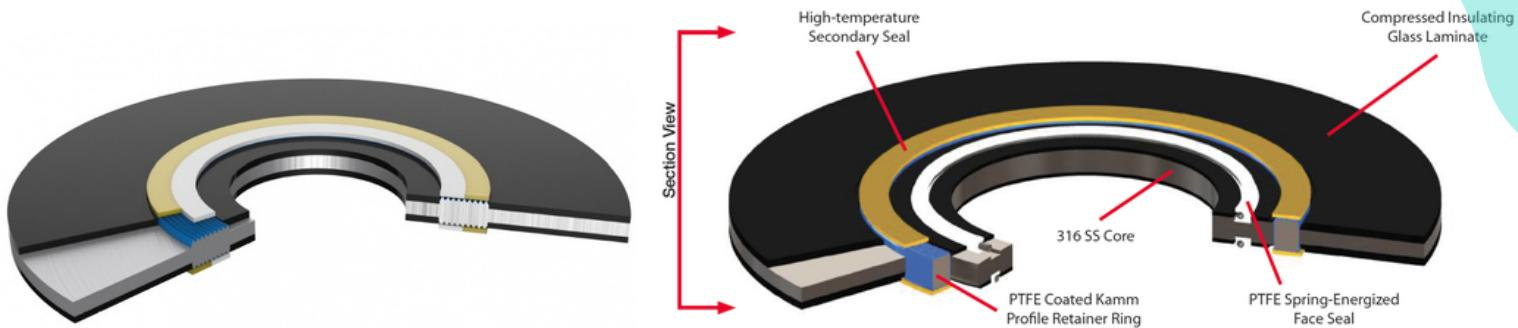
This premium performance fire safe isolation gasket incorporates a coated metallic core housing a modified u-shaped PTFE seal energised with a phynox spring in a patented triple seal design.
